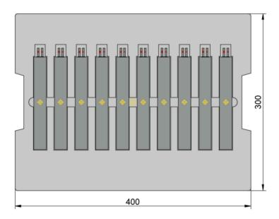
5.2. Cotton box drawing (Tentative) : 15 inner trays / cotton box (max. 150cells / cotton box) Box size : W410mm\*L310mm\*H280mm
