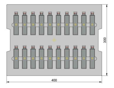
5.2. Cotton box drawing (Tentative) : 15 inner trays / cotton box (max. 300cells / cotton box) Box size : W410mm\*L310mm\*H280mm
